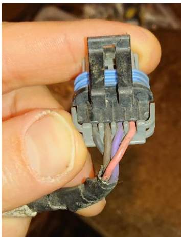
Stock Connector view (only ignition signal color will change)
